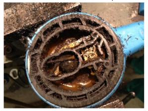
it is only in the inner micro-switch chamber, it means that water got in through the cable thanks to capillary action (see page 1).
