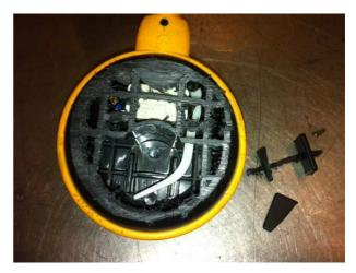
With reference to double chamber float switches like **Supertec** it is necessary to do two cuts.
